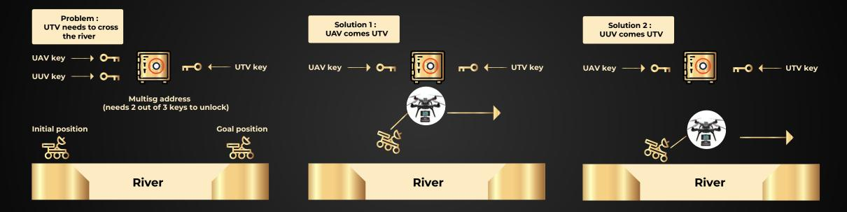
An Unmanned Terrestrial Vehicle (UTV) faces the problem of crossing a river bed. It creates a multisig address in which 2 of 3 keys are needed to establish the collaboration and solve the problem.
