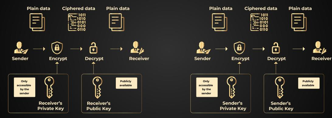
Public key cryptography allows robots to be sure that the content of a message can only be read by the owner of the corresponding sending address.
